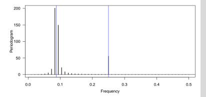
Power at non-Fourier frequencies will leak into the nearby Fourier frequencies
